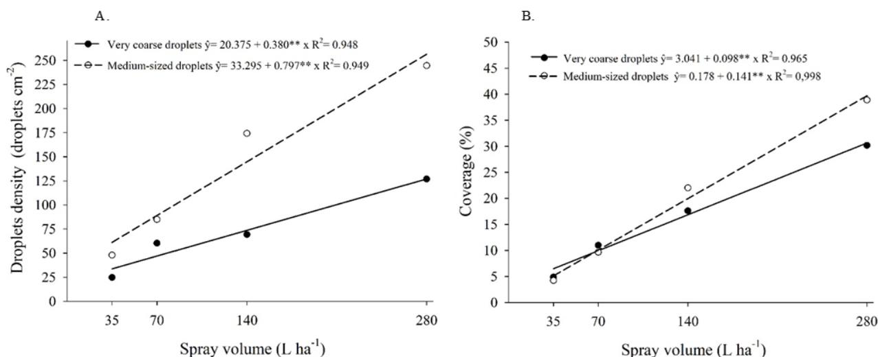
**Figure 2.** Droplet density (droplets  $\text{cm}^{-2}$ ) (A) and coverage percentage (B) in the application of the fomesafen herbicide with an adjuvant (Silwet L-77Ag) using TT11002 spray tip operating at 100 kPa (very coarse droplets) and 400 kPa (medium-sized droplets) according to the spray volume
