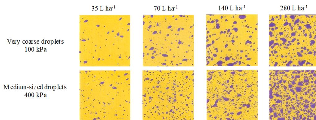
**Figure 3.** Coverage pattern provided by the fomesafen application according to the spray volume and droplet spectrum
