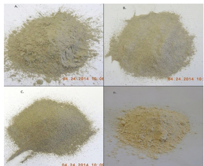
Figure 1. Basalt dusts (A, B and C) with granulometry of 0.1, 0.3 and 0.5 mm, from the municipality of União da Vitória-PR provided by the company Ekosolos Indústria Remineradora de Solos Ltda., and commercial diatomaceous earth (D) (INSECTO ® ) provided by the company Bernardo Química
