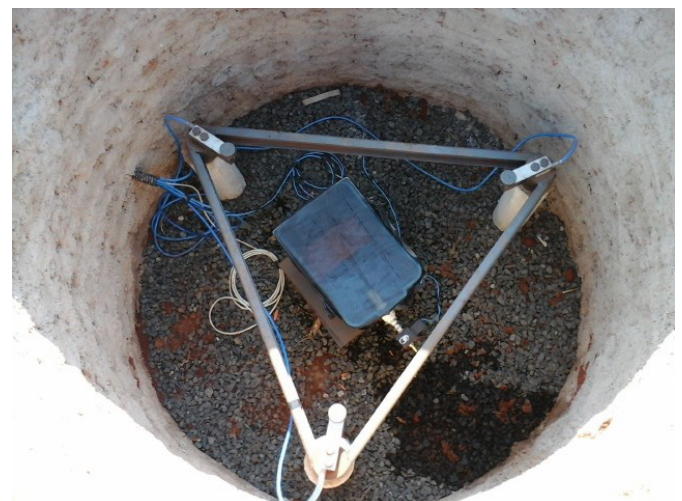
Figure 2. Weighing structure of the lysimeter and drainage system
