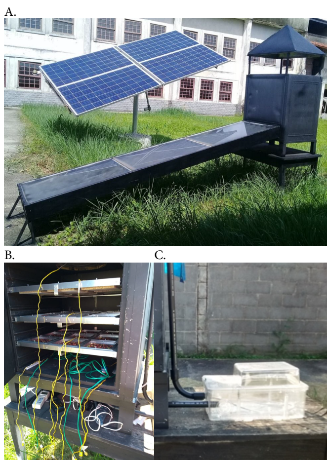
Figure 1. Automated solar drying system: hybrid solar-electric dryer (A), drying chamber (B), acrylic box (C)
