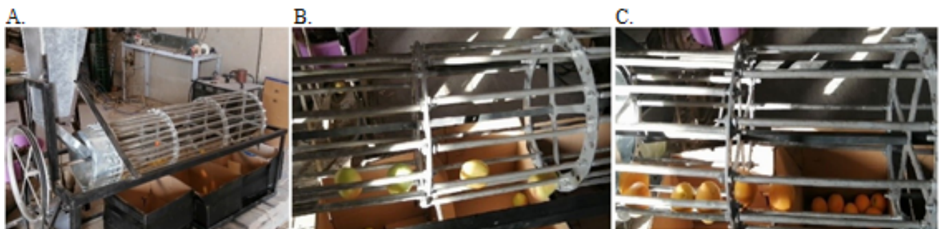
Figure 1. The machine during fruit sorting: (A) Plums, (B) Apples, and (C) Oranges
