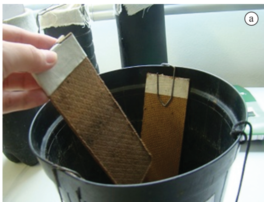
Figura 1. a) Foto de uma ovitampa com duas palhetas, e b) painel frontal do SDP com palheta inserida no sistema. Figure 1. a) Photo of an egg trap with two blades, and b) front panel of the SDP with a palette inserted in the system.
