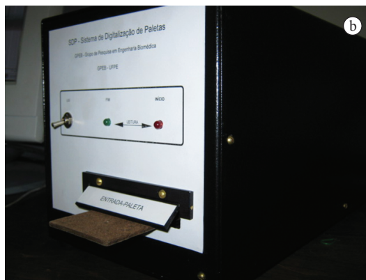
Figura 1. a) Foto de uma ovitampa com duas palhetas, e b) painel frontal do SDP com palheta inserida no sistema. Figure 1. a) Photo of an egg trap with two blades, and b) front panel of the SDP with a palette inserted in the system.
