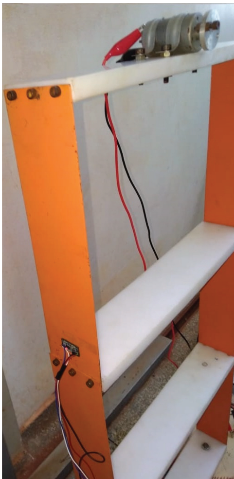
Figure 5: Location of the accelerometer sensor.
