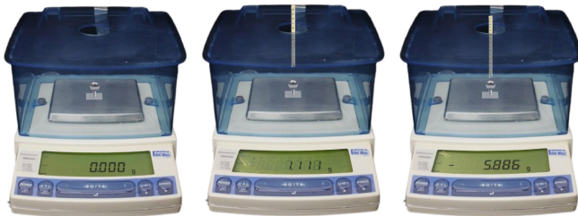
Figure 2: The figure depicts the experimental setup, capturing the shift from repulsion to attraction. In the left panel, the baseline condition shows no second magnet, setting a zero tare on the balance. As the second magnet approaches, the balance records an increase due to a repulsive force (central panel). At closer distances, the force transitions into attraction, indicated by a negative scale reading (right panel). It's important to note that the balance scale readings represent authentic experimental data, while the scaled pen with the magnet at its lower extremity serves as a ruler to measure distance, see also Fig. 3.
