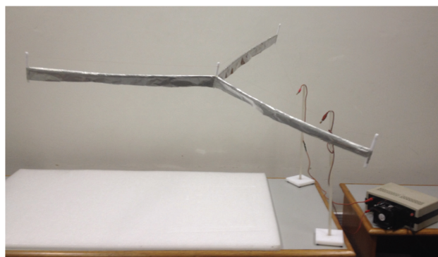
Figura 2 - Lifter (in flight) constructed at the Physics Institute of the University of São Paulo, exhibiting its unique geometry.
