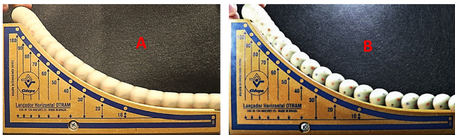
Figure 2: In (A), the sphere’s movement recorded with a trail (blur) is presented. In (B), the sphere’s movement is shown, recorded practically without a trail, and filmed using the video analysis technique by strobe illumination. Notice that the three dots marked on the sphere only appear clearly in (B), while in (A), only in the first few frames is it possible to notice that there is some unsharp marking, then it is no longer possible even to see that the dots are there. Illustration of own authorship.
