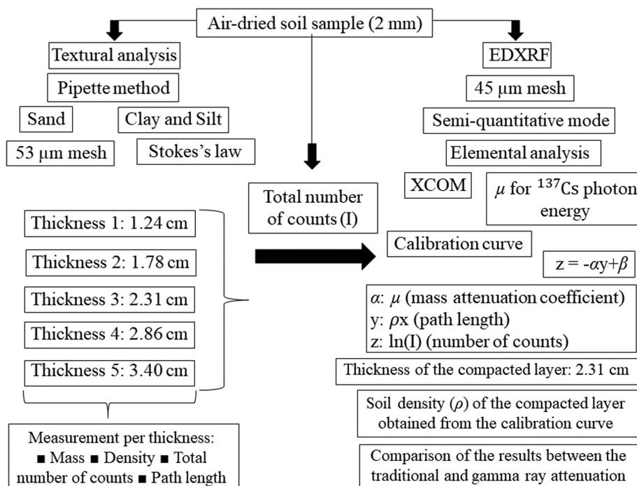
**Figure 3:** Schematic diagram of the procedures carried out in this study.
