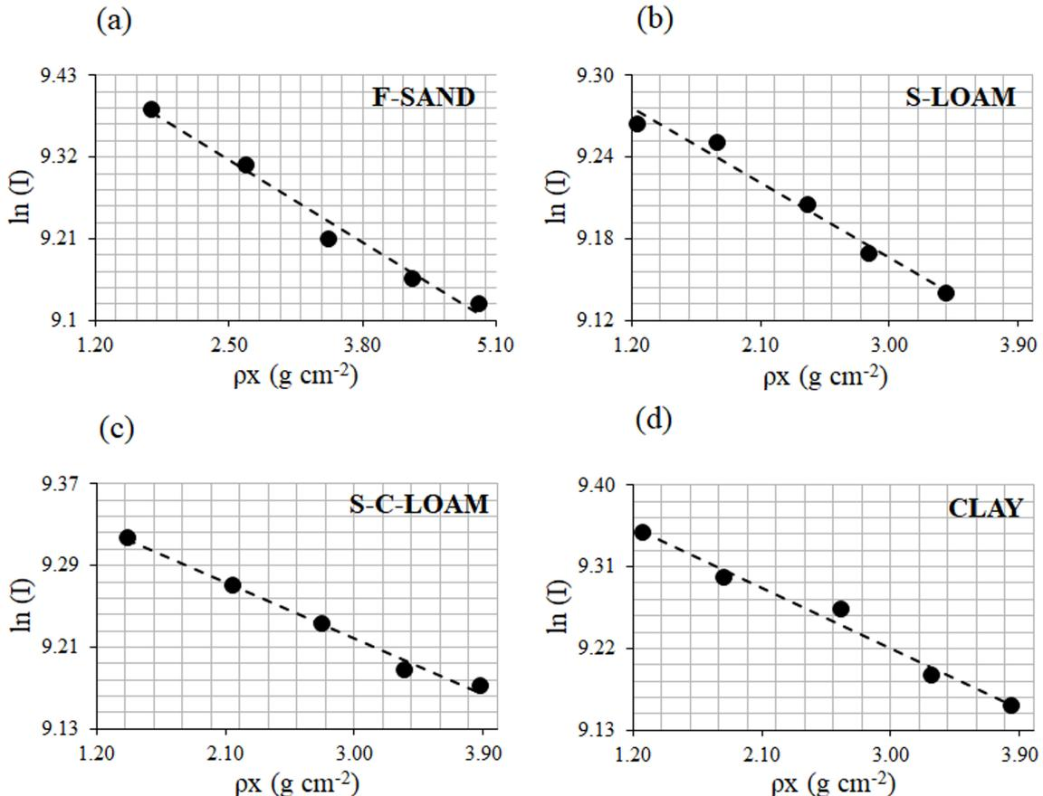
**Figure 5:** Gamma ray photons transmitted  $\ln(I)$  as function of the path length ( $\rho x$ ). (a) F-SAND: Fine Sand. (b) S-LOAM: Silt Loam. (c) S-C-LOAM: Sandy Clay Loam. (d) CLAY: Clay.
