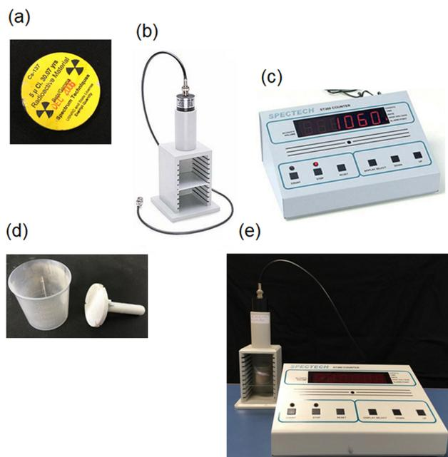
**Figure 2:** (a)  $^{137}\text{Cs}$  educational radioactive source. (b) Student Geiger-Müller (GM) tube. (c) Radiation counter system. (d) Sample container and pestle. (e) View of the experimental setting up.
