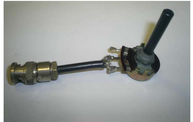
Figure 3 - A potentiometer of 1 k \Omega used in shunt with the oscilloscope.
