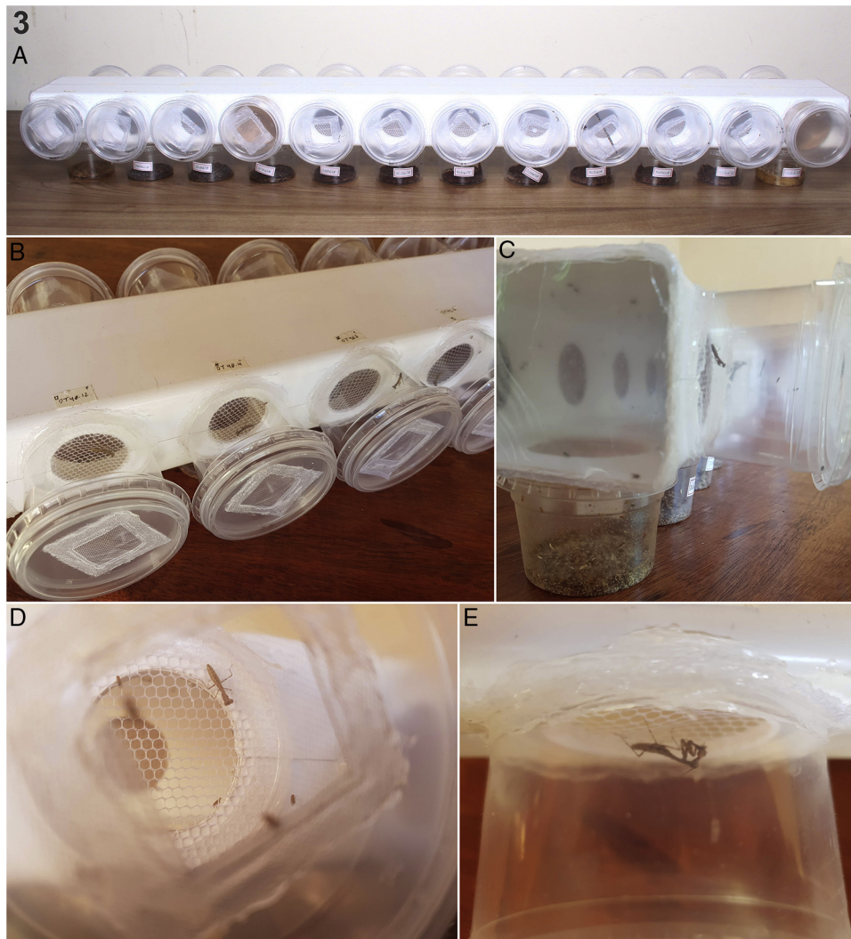
Fig. 3. Model B autofeeder in operation. (A) Overall view; empty rearing chambers have a cardboard disk blocking the entrance of flies. (B) Four 4th and 5th instar M. aptera Giglio-Tos, 1917 in the rearing cups along with some Drosophila Fallén, 1832 flies. (C) Front view of one end of the equipment, showing the prey cup with culture medium, and Drosophila larvae and flies; note central compartment with prey freely circulating, and the rearing cup with a 4th instar M. aptera hanging in the Tulle fabric. (D) Rearing cup seen through its cover lid, with a 4th instar M. aptera and some prey. (E) Side view of the rearing cup, with a 5th instar M. aptera feeding on a freshly caught Drosophila fly.
