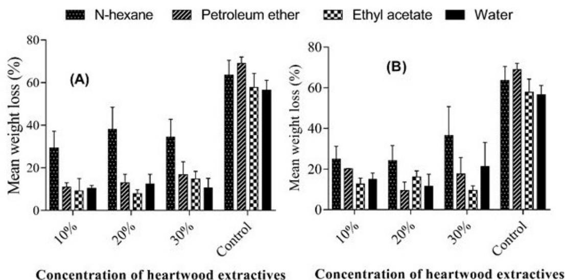
**Figure 2.** Comparison of mean weight loss (%) of *P. deltooides* wooden stakes dipped in different concentrations of n-hexane, petroleum ether, ethyl acetate and water solvents based *Z. mauritiana* heartwood extractives for 36 (A) and 72 (B) hours after exposure to termites.
