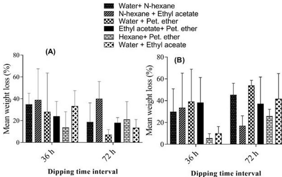
**Figure 4.** Comparison of mean weight loss of *P. deltooides* wooden stakes dipped for 36 h and 72 h in 30% concentrations of different mixture of *Z. mauritiana* heartwood (A) and bark (B) extractives
