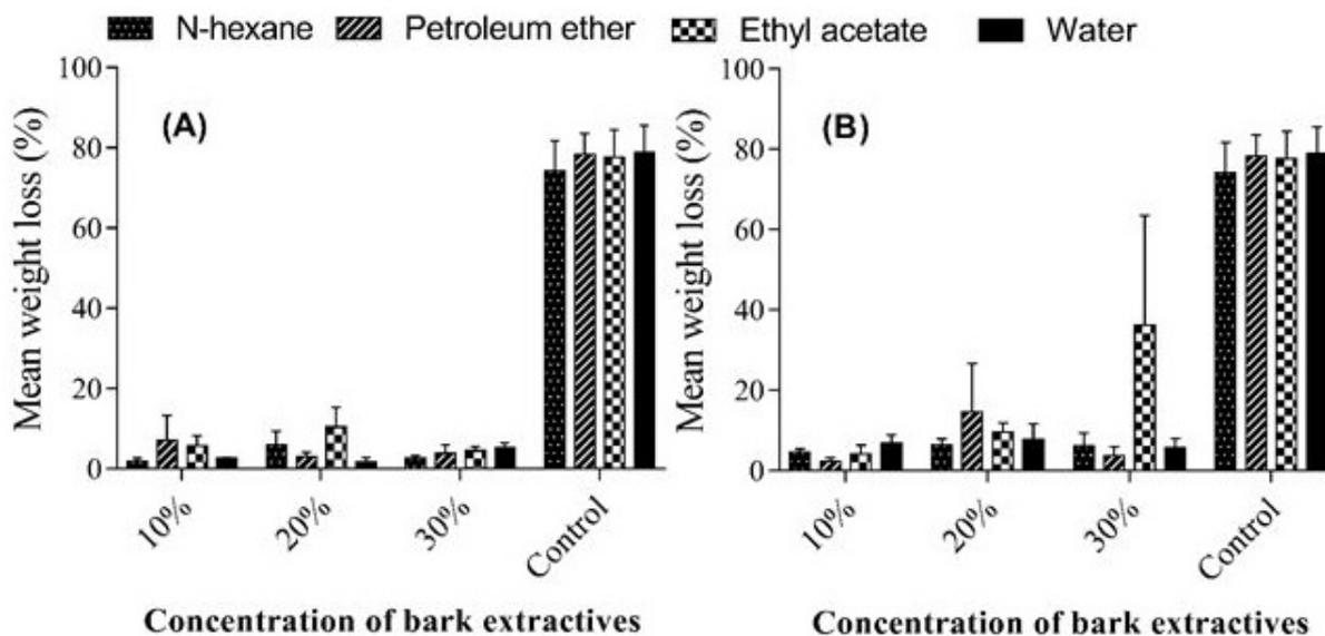
**Figure 3.** Comparison of mean weight loss (%) of *P. deltooides* wooden stakes dipped in different concentrations of n-hexane, petroleum ether, ethyl acetate and water solvents based *Z. mauritiana* bark extractives for 36 (A) and 72 (B) hours after exposure to termites.
