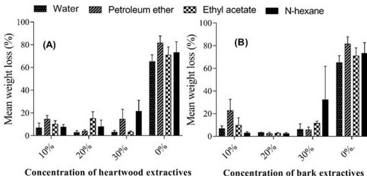
**Figure 5.** Comparison of mean weight loss of *P. deltooides* wooden stakes oven dried at 80°C for seven day and treated with different concentrations of *Z. mauritiana* heartwood (A) and bark (B) extractives by dipping for 72 h.
