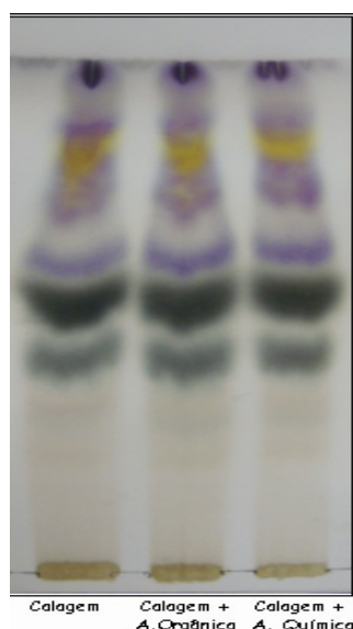
Figure 6. Chromatographic profiles of the flowers of calendula subjected to different treatments. Stationary phase: silica gel (FG 254 ). Mobile phase: Merck® mixture of anhydrous formic acid:glacial acetic acid:water:ethyl acetate (11:11:27:100 v/v), methanolic solution of 5% sulphuric acid (v/v) followed by 1% sulphuric vanillin (v/v).
