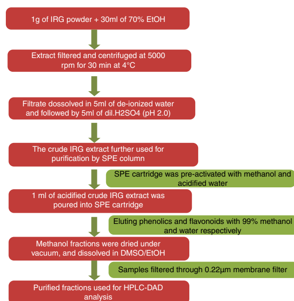
Fig. 1. Flowchart illustrating the extraction and separation of phenolics acids and flavonoids in Lolium multiflorum sample.
