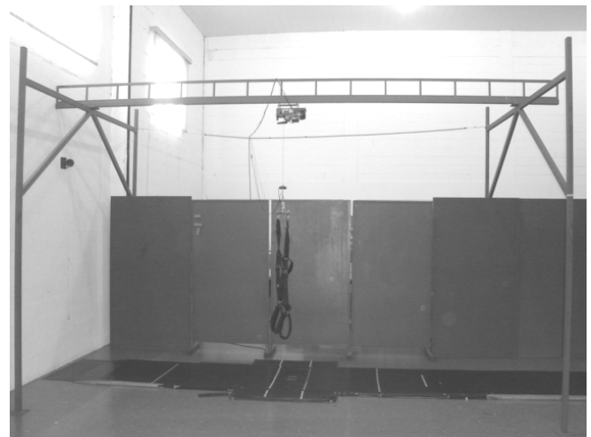
Figure 1. Partial view of experimental setting, showing the walkway, metal structure, motor and vest.
