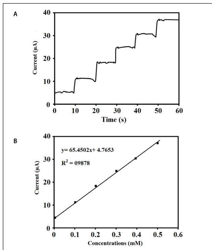
**Figure 3.** (A) The amperogram of Au@CNTs/GCE into 0.1M PBS of various levels of lactate into real samples; (B) graph of the calibration curve.
