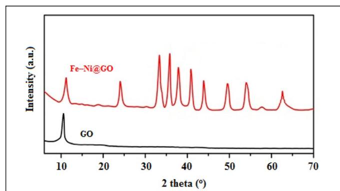
Figure 2. XRD patterns of prepared GO and Fe-Ni@GO.
