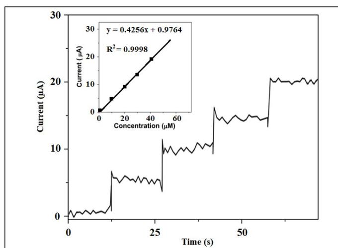
**Figure 4.** Amperometric analysis and calibration curve of Fe-Ni@GO/GCE to consecutive adding 10  $\mu\text{g}/\text{ml}$  insulin into prepared blood samples at 0.1V.
