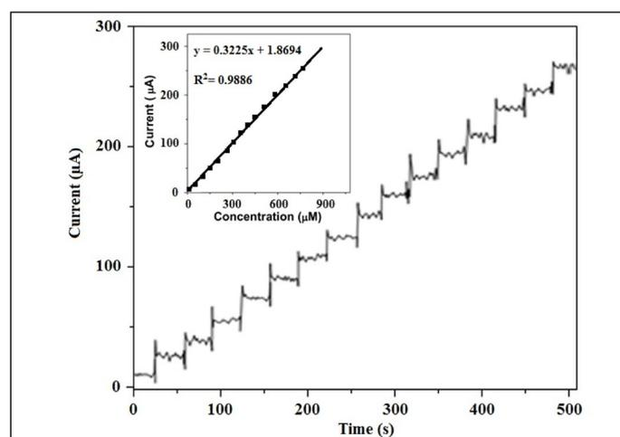
**Figure 3.** Amperometric analysis and calibration curve of Fe-Ni@GO/GCE to consecutive adding 100  $\mu\text{M}$  insulin into 0.1M PBS at 0.1V.
