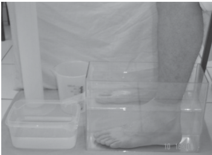
Fig. 1 – Volumetric measurement: A) volumeter, B) recipient, C) test tube, D) Becker flask.
