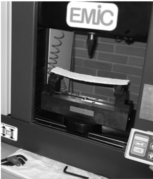
Fig. 3 - Flexion test at three points.
