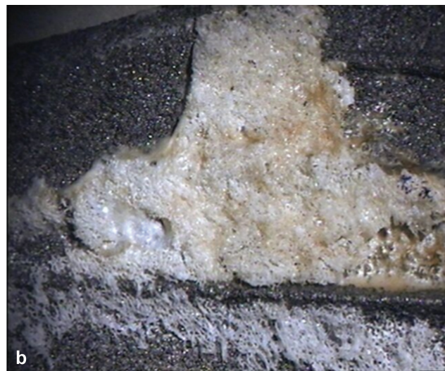
Fig. 2 Photographs of a Logical stem removed due to infection. The images show clear bone growth at the porous surface of the stem.
