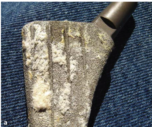
Fig. 2 Photographs of a Logical stem removed due to infection. The images show clear bone growth at the porous surface of the stem.
