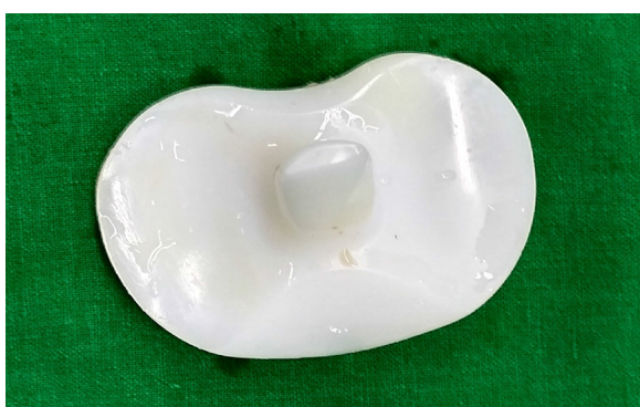
Fig. 4 – Image of the superior surface showing lack of any deformation on the articulating side, including the post.
