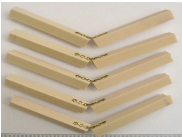
Fig. 7 – Illustrative photo of group I after the mechanical test.
