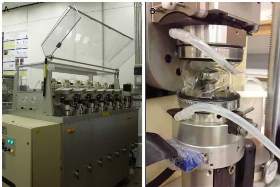
Fig. 1 – (A) General view of a hydraulic multi-station hip simulator; (B) detail of a work station with a hip joint test specimen (without lubricant).
