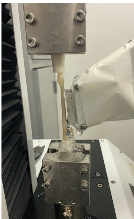
Fig. 7 Transducer positioning during testing on the traction machine.
