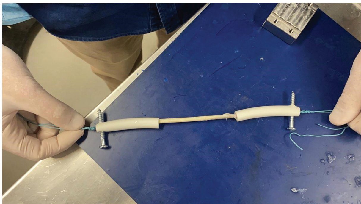
Fig. 3 Semitendinosus tendon (ST) inserted into tubes and fixated to the framework with screws.
