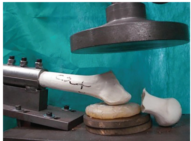
Fig. 3 Synthetic bone after the mechanical test. A basicervical fracture is noted in this specimen.
