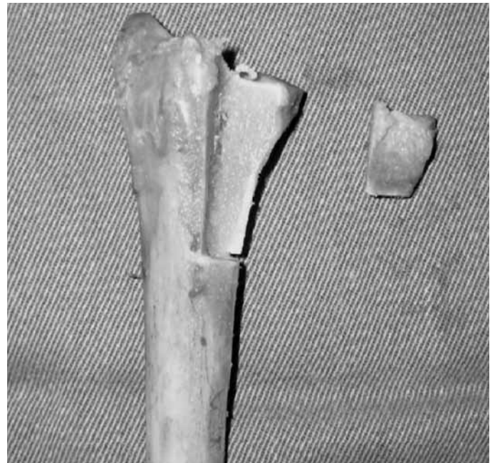
Figure 2 – Photograph of the dorsal face of the distal region of the radius, demonstrating the bone failure and the distal fragment that separated.
