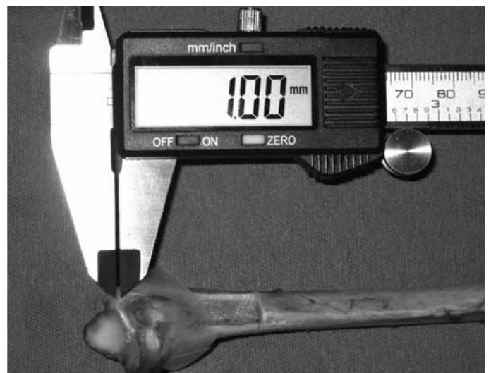
Figure 3 – Joint step of 1 mm, measured using digital calipers, and bone fragment fixed with colorless adhesive tape.
