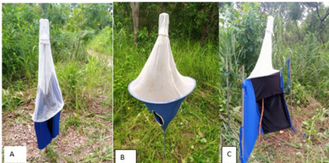
Figure 2. Traps used in seasonal monitoring of tsetse flies: (A) Vavoua trap, (B) Biconical trap, and (C) NGU trap, in The Gambia.
