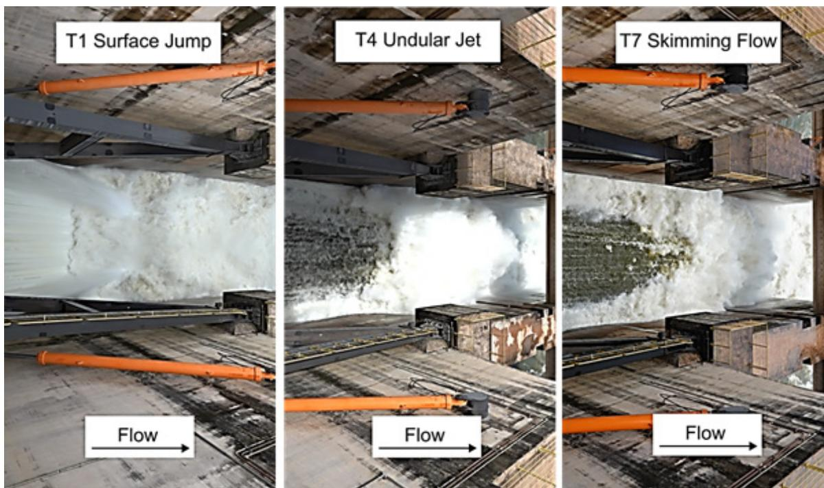
Figure 12. Spillway jet regimes – Top view of spillway bay.
