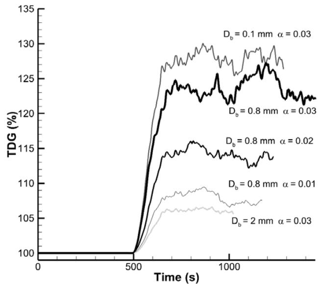
**Figure 8.** Average TDG at the model downstream end for the sensitivity analysis simulations.
