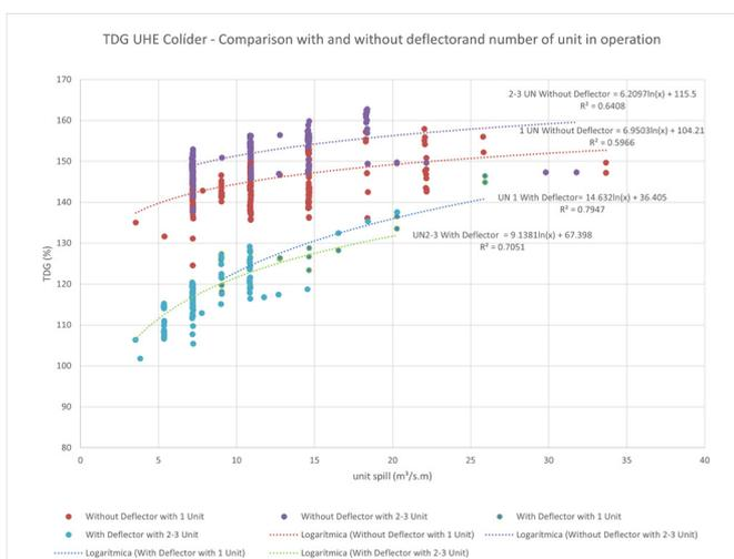
**Figure 14.** TDG concentration in the stilling basin with and without deflector with powerhouse flows.
