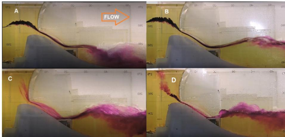
Figure 3. Jet regimes in the physical reduced-scale model: (A) Plunging flow (B) Skimming flow (C) Undular Jet (D) Surface Jump.
