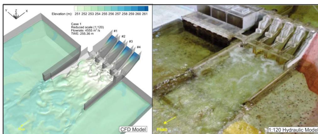
**Figure 6.** Free surface characteristics in the tailrace for Case 1. Top: CFD and bottom: 1:120 hydraulic model.
