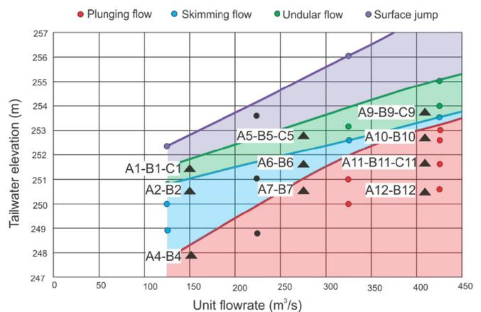
**Figure 10.** Simulation conditions to evaluate the deflector elevation and spillway jet regime observed in the 1:60 scale hydraulic model.
