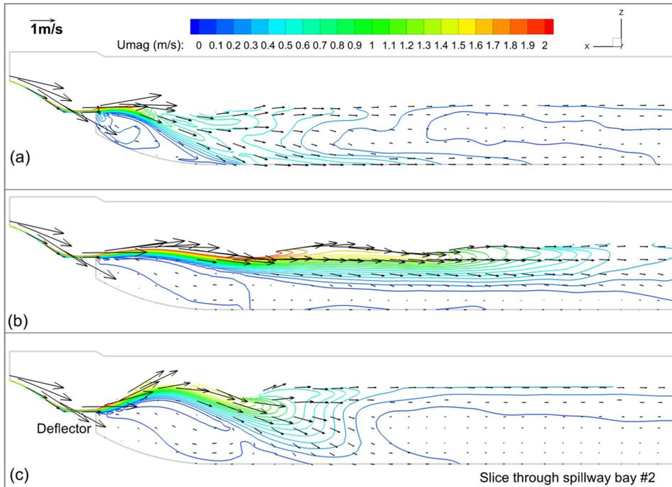
**Figure 7.** Spillway jet regimes. (a) plunging at TWE 248.8 m, (b) skimming at 251.0 m, and (c) surface jump at TWE 253.5 m.
