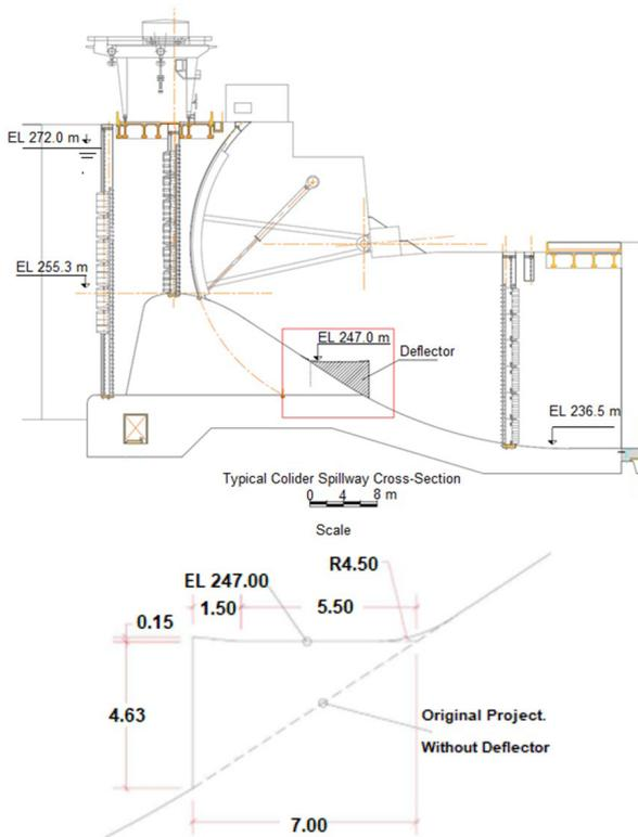
Figure 2. Colider spillway cross-section with deflector.
