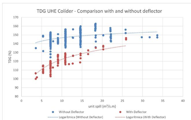
**Figure 13.** TDG concentration in the stilling basin with and without deflector without powerhouse flows.
