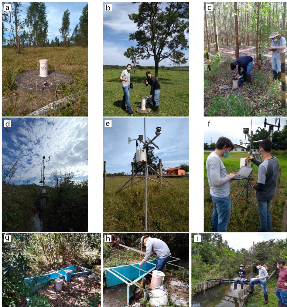
Figure 6. Images of the OCW instrumentation and the monitoring team working: (a) Well 19 (P19 at Figure 2); (b) Well 26 (P26 at Figure 2) with manual level verification in progress; (c) Well 9 (P9 at Figure 2) with manual level verification in progress; (d) Riparian Zone Automatic Meteorological Station (EM-ZR at Figure 2); (e) Monte Alegre Automatic Meteorological Station (EM-MA at Figure 2); (f) Santo Ignacio Automatic Meteorological Station (EM-STO at Figure 2) with data collection in progress; (g) Parshall Flume 1 (Q1-CP1 at Figure 2); (h) Parshall Flume 2 (Q2-CP2 at Figure 2); (i) Santa Maria da Fábrica stream gauge (Q3-SMF at Figure 2), with a hydrometric current-meter in use.
