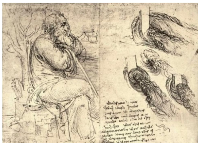
Figure 1. Leonardo da Vinci's drawing of turbulent free surface flows around obstacles. Richter (1883, Part I, p. 200).
