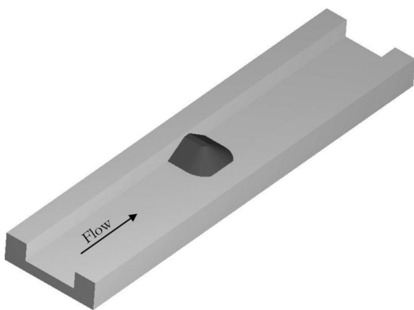
Figure 14. Channel and cofferdam in a computational model.
