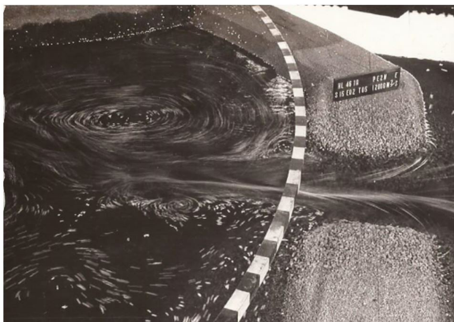
Figure 4. Hydraulic scale model study of the Paraná river closure to build the Itaipu Hydroelectric Plant. Source: CEHPAR (1976).
