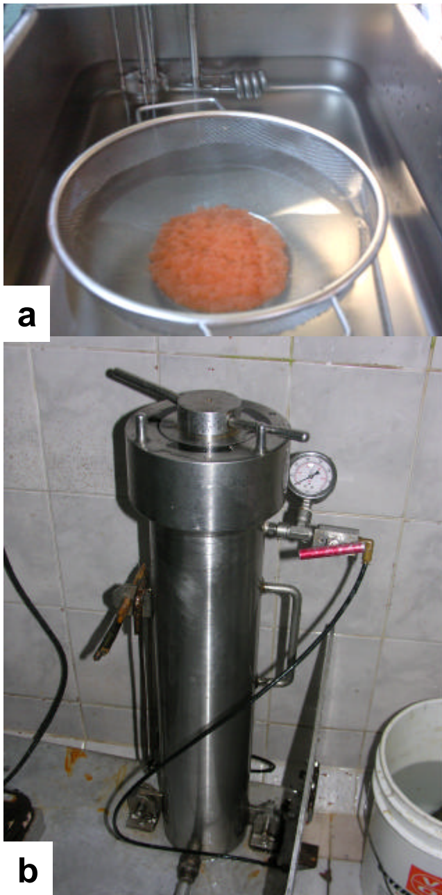
Figure 2 - a) thermic shocks application to recently fertilized eggs from rainbow trout ( Oncorhynchus mykiss ) b) pressure system for triploidy induction.
