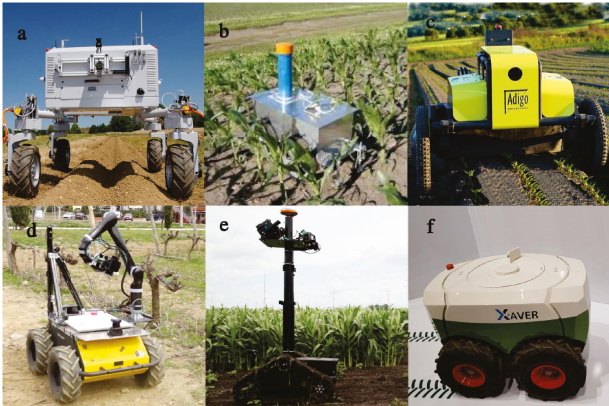
Figure 2 - Displays some examples of robots with rigid suspension
