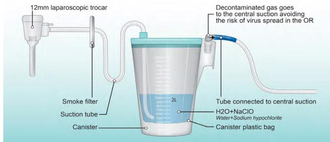
**Figure 2.** Diagram of the pneumoperitoneum filtration system improved with common OR equipment.
