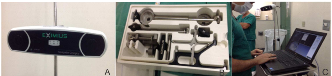
Figure 3 - Components of the Eximius system: A) camera; B) instruments; and C) computer with navigation platform.
