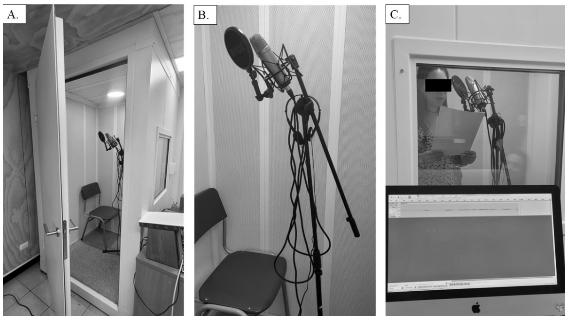
Figure 1. Equipment used for the audio recordings at the USACH Phonetics Lab. A. Soundproof booth; B. Microphone model RØDE NT1-A; C. Audio recording using the software Audacity version 3.1.3. for Mac.
