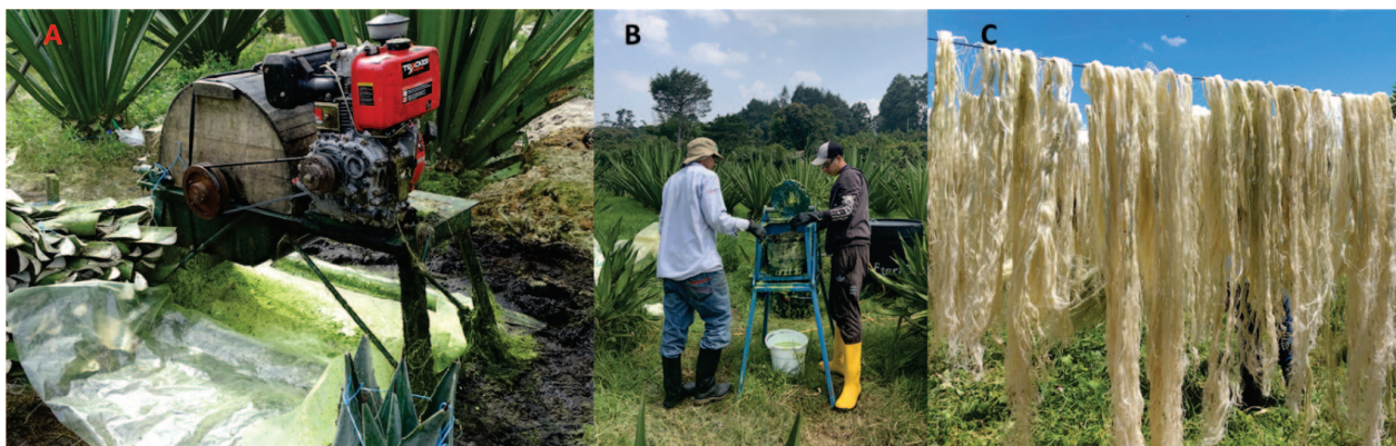
Figure 1: Figue fiber extraction process ( Furcraea spp.) in Rionegro, Antioquia, Colombia. A. Traditional machine used. B. Biomass separation system. C. Fiber drying. Photographs: A. Medina C., B. Orozco L, C. Grisales N.
