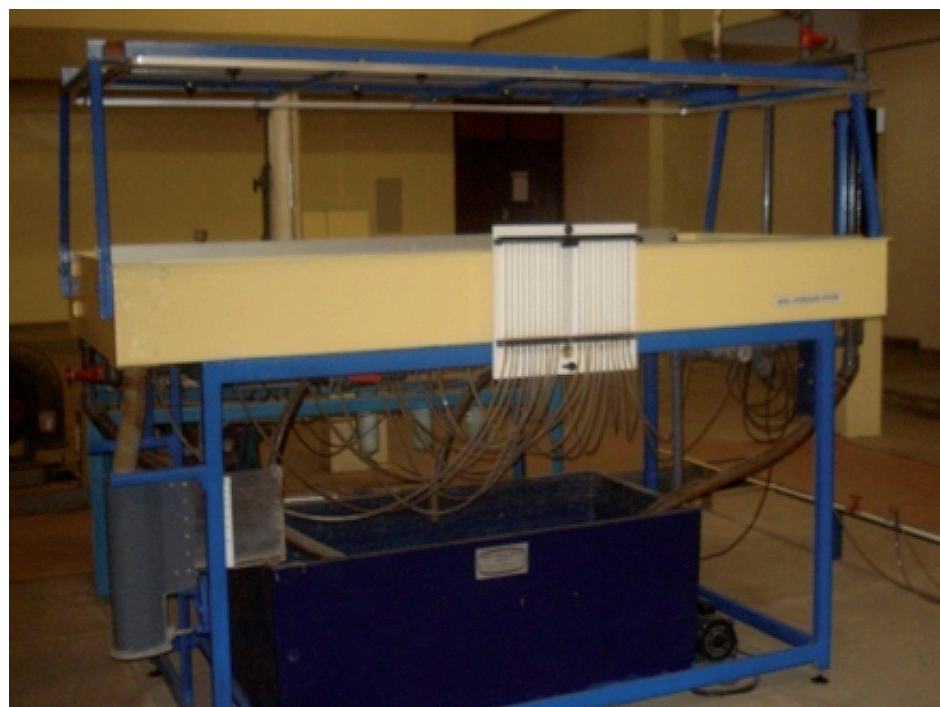
Figure 1 Equipment utilized for rainfall simulation
