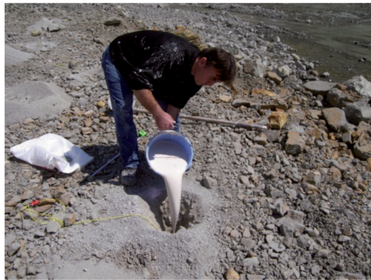
Figure 4 Pouring of plaster paste into hole collar.
