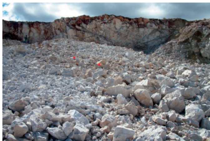
Figure 7 Rock pile from blast round with drill cuttings stemming at Gumusgun limestone quarry.
