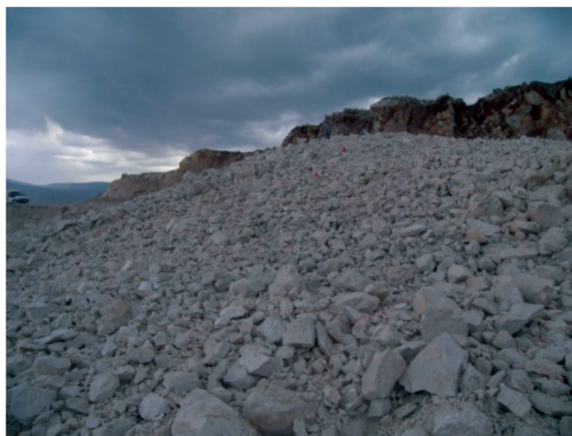
Figure 8 Rock pile from blast round with plaster stemming at Gumusgun limestone quarry.
