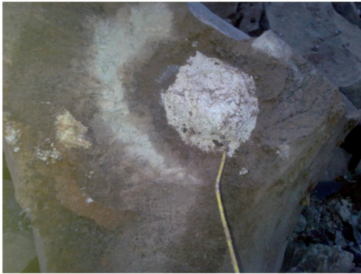
Figure 2 A plaster plug is not ejected from the hole during explosion at a basalt quarry.
