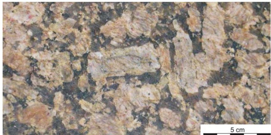
Figure 4 - Porphyritic granite with cumulative large phenocrysts of an ornamental rock of unknown commercial name, sample THOR1.
