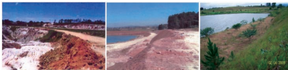
Figure 1 São Caetano pit at operation (L), decommissioning in 2003 (M) and under rehabilitation in 2009 (R).
