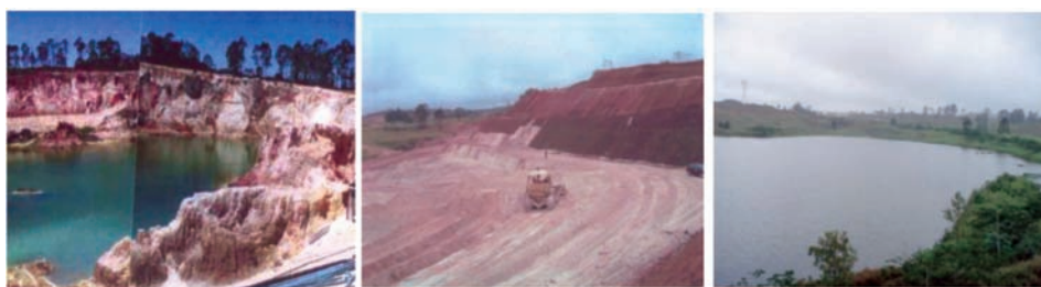
Figure 2 Bianchi pit at operation (L), decommissioning in 2003 (M) and under rehabilitation in 2009 (R).
