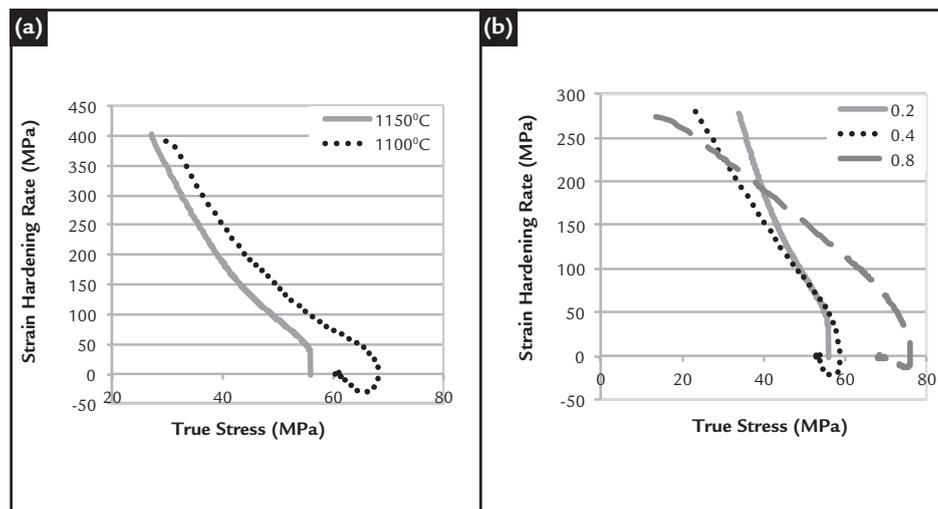
Fig. 4 Strain Hardening Rate Variation ( $\theta$ ) versus True Stress for API 5L X80 steel: (a) for different temperatures at a constant strain rate 0.2s<sup>-1</sup>. (b) for different strain rates and a constant temperature of 1150°C.
