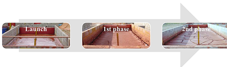
Figure 10 - Generation of the dry cracks mosaic. Source: Pedrosa (2012).
