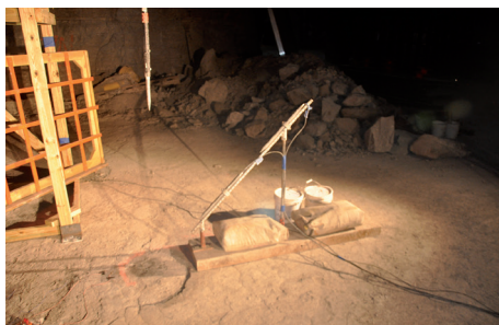
Figure 3 Typical Pencil Pressure Sensor Array.
