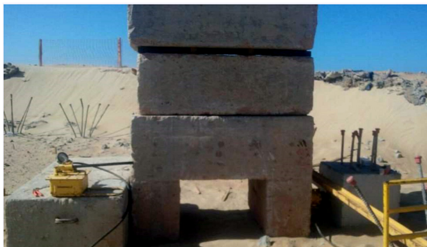
Figure 3 – Horizontal load test performed in loco .
