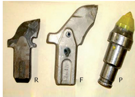
Figure 1 (R)Radial, (F) forward attack and (P)point attack picks, (Eyyuboğlu, E.M, 2000).
