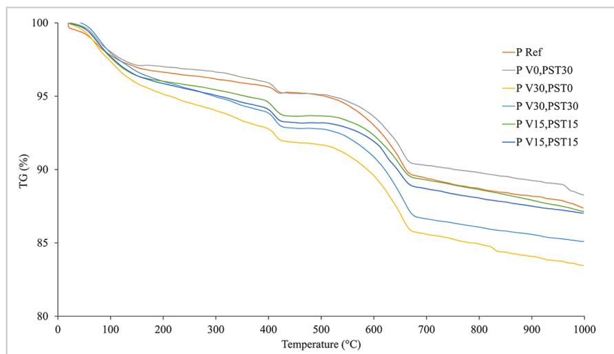
Figure 3 - Thermogravimetry (TG) of ground paver waste.
