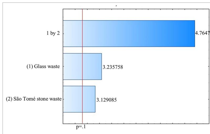
Figure 5 - Pareto chart of factors (1) Glass waste, (2) São Tomé stone waste and 1 by 2 for water absorption after 50 days.
