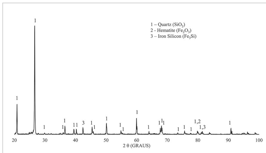
Figure 1 - Diffractogram obtained from the São Tomé stone waste.
