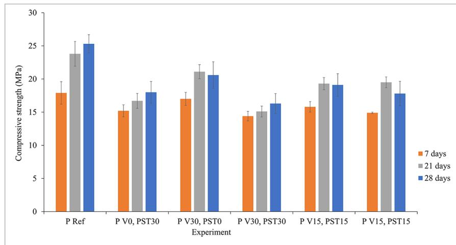
Figure 7 - Compressive strength of paver samples at 7, 21 and 28 days.
