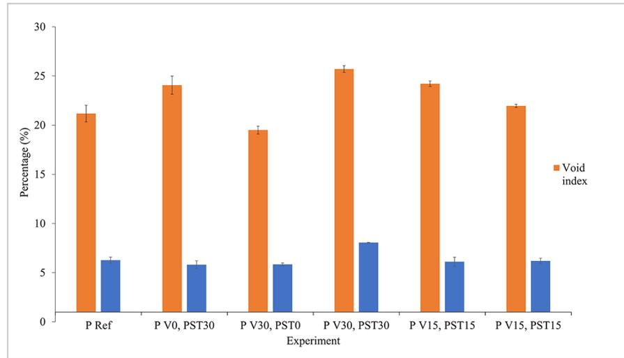
Figure 4 - Water absorption and voids index (Iv) of different paver compositions.
