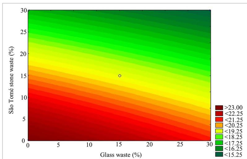
Figure 9 - Response surface graph for compressive strength of the pavers containing São Tomé stone waste and glass waste after 21 days.
