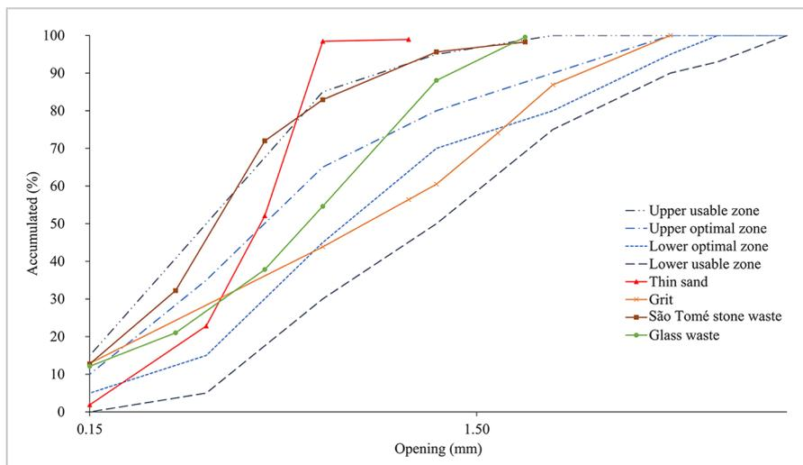
Figure 2 - Distribution of granulometric composition and limits established by the standard.
