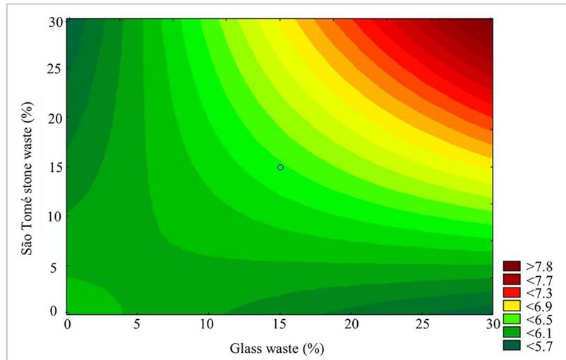
Figure 6 - Response Surface graph for water absorption of the pavers after 50 days.
