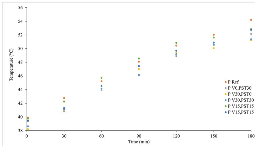
Figure 11 - Thermal representation of the pavers subjected to sunlight radiation.
