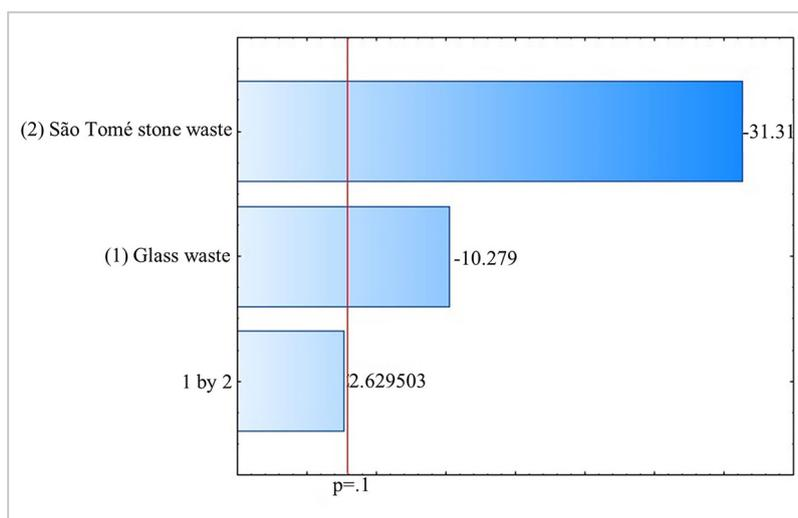
Figure 8 - Pareto chart of factors (1) Glass waste, (2) São Tomé stone waste and 1 by 2 for compressive strength after 21 days.
