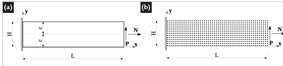
Figure 3 - Cantilevered beam under axial and transverse load: (a) geometry; (b) model discretized in field nodes.
