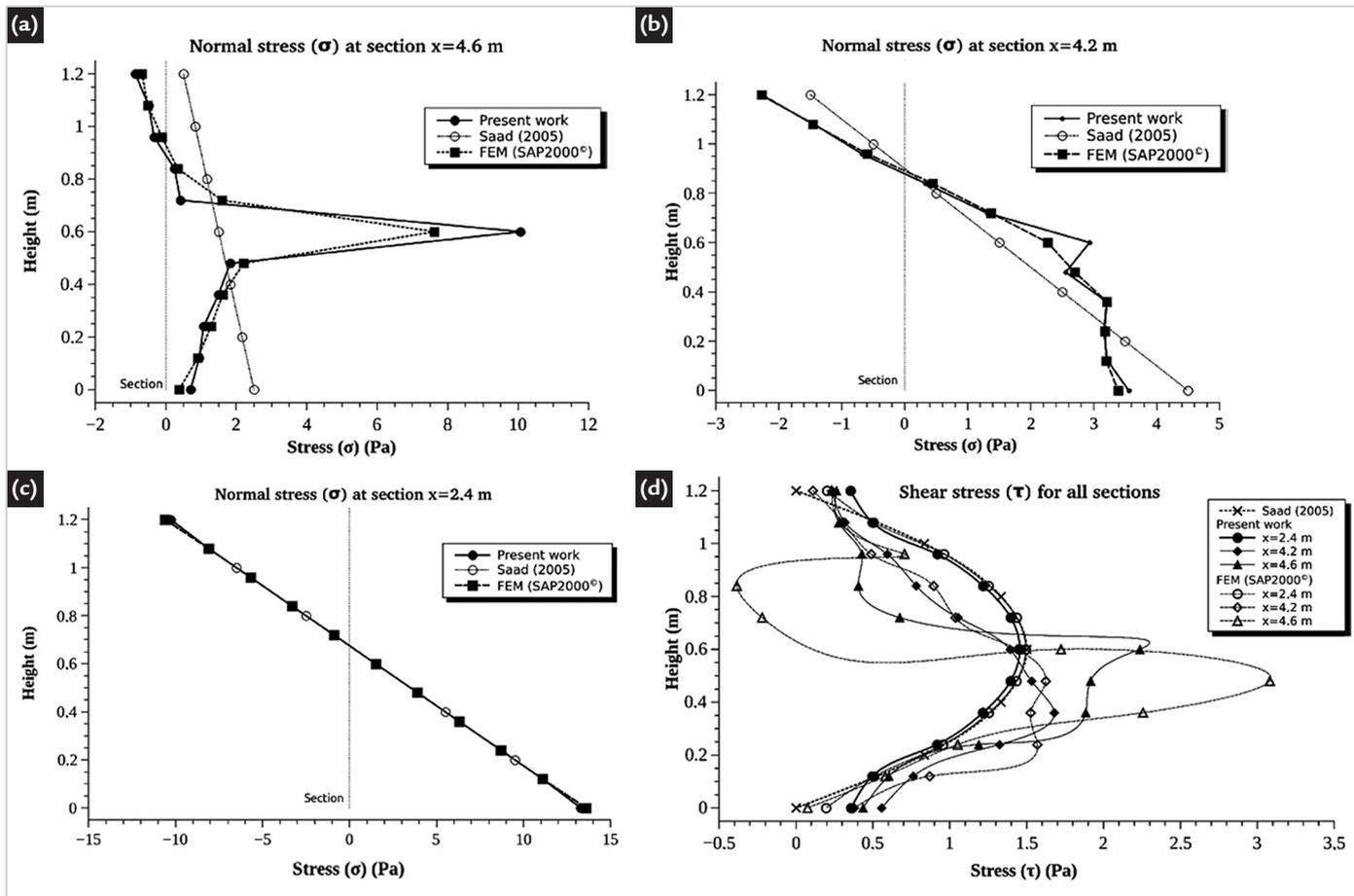
Figure 4 - Numerical and analytical results for example 2: (a) normal stress at  $x=4.6\text{m}$ ; (b) normal stress at  $x=4.2\text{m}$ ; (c) normal stress at  $x=2.4\text{m}$ ; (d) shear stress for all sections.
